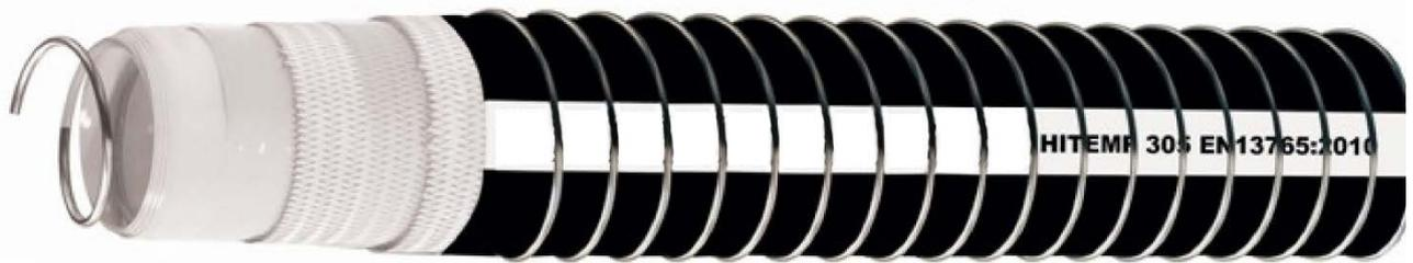
**HITEMP 305** is a multi-layer thermoplastic hose designed around several fluoropolymer liners, supported by a stainless steel inner wire and reinforced with films and fabrics specifically designed for high temperature applications. All the different layers are wrapped together and tensioned between internal and external wire spirals.
